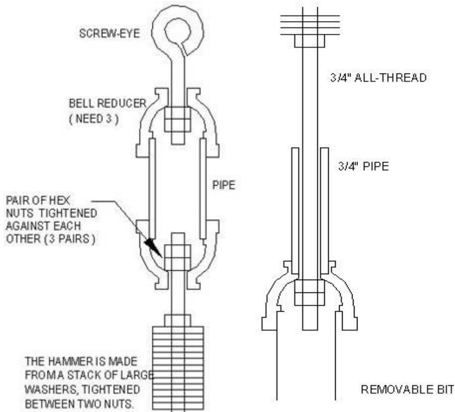
Periodically, the assembly is withdrawn, and the section below the 1-1/4" coupler is removed and emptied.
