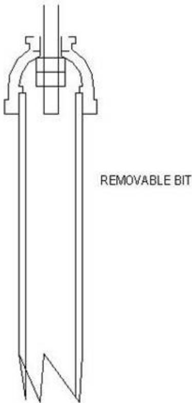
I made a bit for removing loosened soil and thick mud by threading a carriage-bolt through the bit and a couple of sheet-metal flaps, a couple inches above the bottom.
