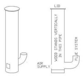
I made my first version of this from a 5" diameter piece of sheet-metal pipe, about 30" long. I used 3" pipe for the flue. Use at least 10' of flue to develop a satisfactory draft
