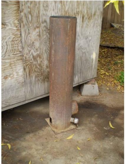
The air inlet is at the bottom on the left, and the 6" flue connection is at the lower right. The capped pipe at the bottom right has a mate on the other side. This option allows extra air right at the exit point, to help keep the flue entrance free of ash.
