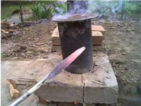
Rather than worry about the status of the air flow, I fitted the opening with a rectangular tube 5" wide by 1-1/2" high, by 4" long. I then screwed a weighted bolt through a 6"-long steel strap, and attached a metal flap as shown below.
