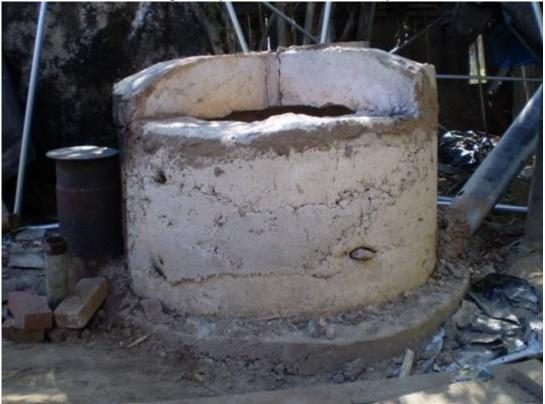
The fire box is an 8" pipe that feeds the wood vertically into a small intense fire at its base. The principle and technology of this style is detailed in the section titled "Basic Stove".
