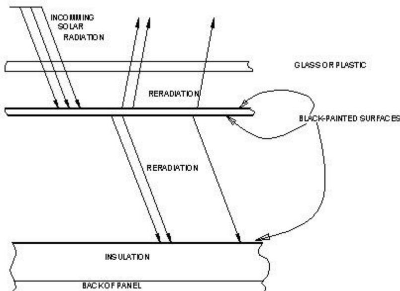
This way, about half of the re-radiated energy is sent deeper into the panel, where it is reabsorbed.
