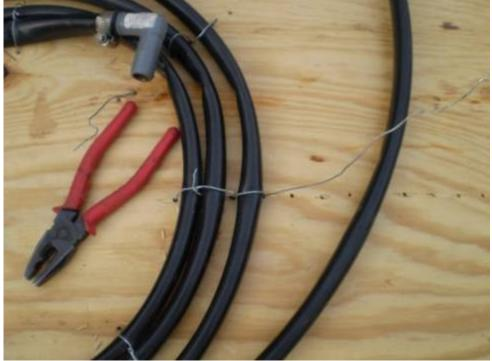
In this case, the plywood is used only as a workbench, and is not actually attached to tubing. The tubing is connected only to itself as the wires are simply woven back and forth to capture each winding in several places. Additional sections of wire lacing might be added to the outer turns to give more
