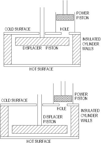
Referencing the drawing left, the energy is obtained from the temperature difference between the COLD SURFACE and the HOT SURFACE. These two surfaces are separated by a cylinder of an insulating material so that the two surfaces will not cancel each other out by conduction.
