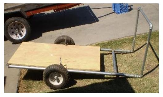
In this next case, this same pair of wheels is attached in the same manner to a three-wheel frame. This type of flexibility lends itself to a wide range of experimentation.
