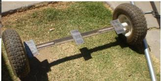
Steel pads were welded to the assembly to aid in attaching a chassis. This chassis was a simple frame welded up from electrical conduit. A separate handle was made from standard plumbing pieces, and made detachable so the whole thing could be tossed into the trunk of a car if need be.
