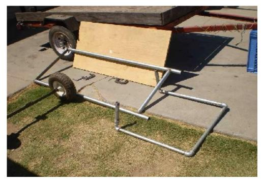
The chassis in this case is attached to the pads on the axle by a couple of "C" clamps that sandwich it between the plywood deck and the pads provided on the axle assembly.
