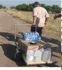
This photo shows a custom hand cart being used to haul bottled water for a homeless community. An axle was made by cutting off the heads of bolts and welding them thread-ends out to a piece of angle iron. Wheelbarrow wheels were then added to the protruding ends and secured with locking nuts. Since each of these wheels typically have a load rating of 300 pounds or more, this axle assembly has a lot of potential.
